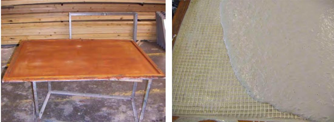
Figure 4 Mould and test board casting
