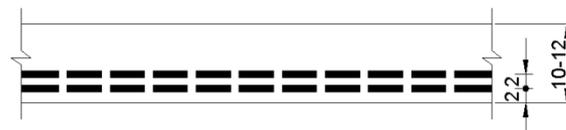
Position of glass fibre mesh in the board
