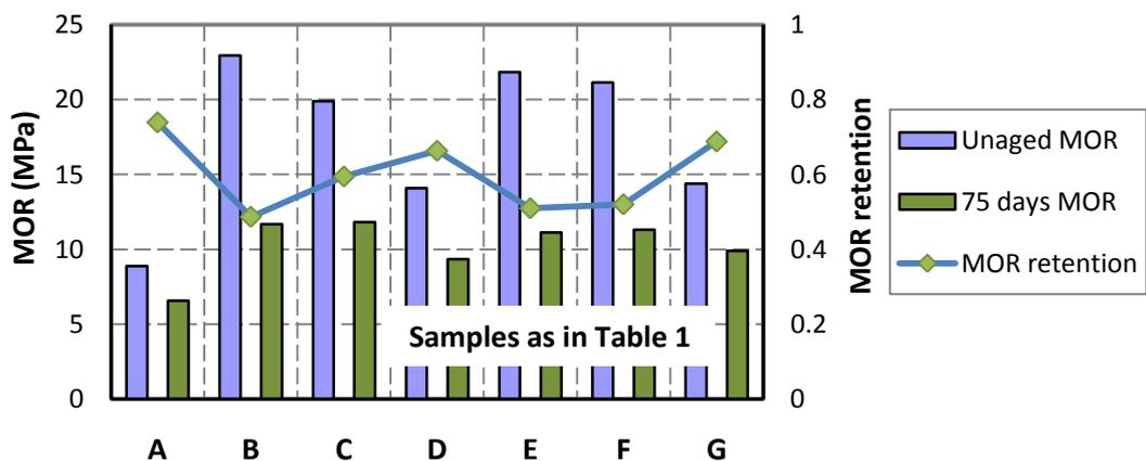
**Figure 6 Residue MOR after 75 days accelerated ageing**
