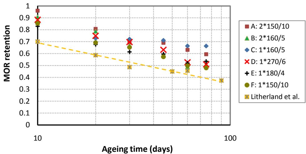
**Figure 9 Fibre mesh reinforced GRC ageing performance**
