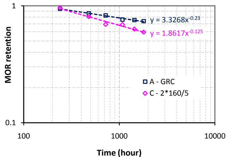
Figure 16 MOR retention vs. time and  $R_{10}$
